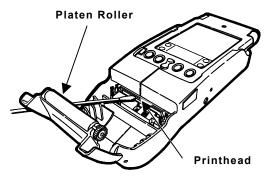
4. Clean the platen roller with a dry cloth or small brush. You can also use a cotton swab moistened with isopropyl alcohol. Turn the platen roller with your finger and run the cotton swab or dry cloth across it. Make sure the platen roller is clean all the way around.
